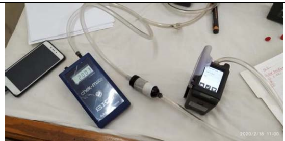
Figure 4 - Calibrating the pump before sampling
